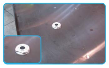
Install the supply fitting as shown. This includes a second low profile nut and white rubber washer. There should be no exposed threads on the interior surface of the lid per NSF guidelines.
