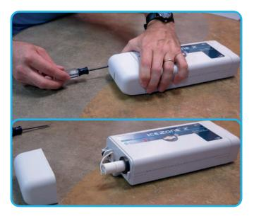
Remove the service cover from the ICEZONE unit. This provides access to the lamp, power input and mounting boss. As the screw is removed from the cover, be sure to keep it with the cover so it is available for re-assembly.
