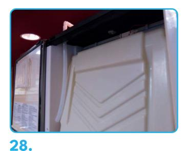
Test the movement of the ice curtain to ensure proper operation. The return tube should not prevent the curtain from activating the "bin full" switch.
