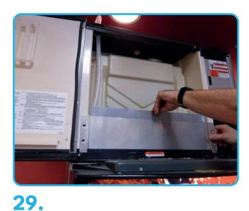
Replace the ice shield and sanitize this as well before turning the ice machine on and closing the cover.
