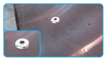
Install the supply fitting as shown. This includes a second low profile nut and white rubber washer. There should be no exposed threads on the interior surface of the lid per NSF guidelines.
