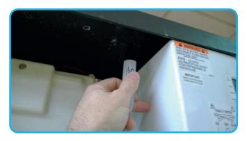
Mark the location for the ICEZONE return fitting. This is the fitting where the plasma will return to the ICEZONE. This should be located on the right side of the top cover (looking at the front of the ice machine). This hole should be spaced off of the interior wall of the ice machine by 2.0 inches. The hole should be spaced from the front edge of the ice machine cover by 2.0 inches also.
