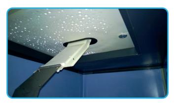
Install the return fitting as shown. This includes a second low profile nut and white rubber washer. There should be no exposed threads on the interior surface of the lid per NSF guidelines.
